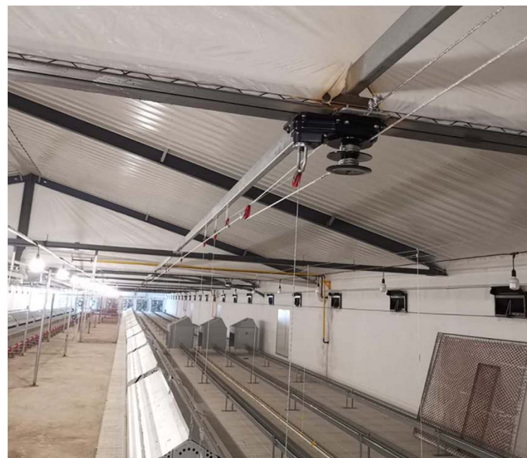
Equipped with egg box lifting system, cleaning hen house and brood rearing period without disassembling egg box
