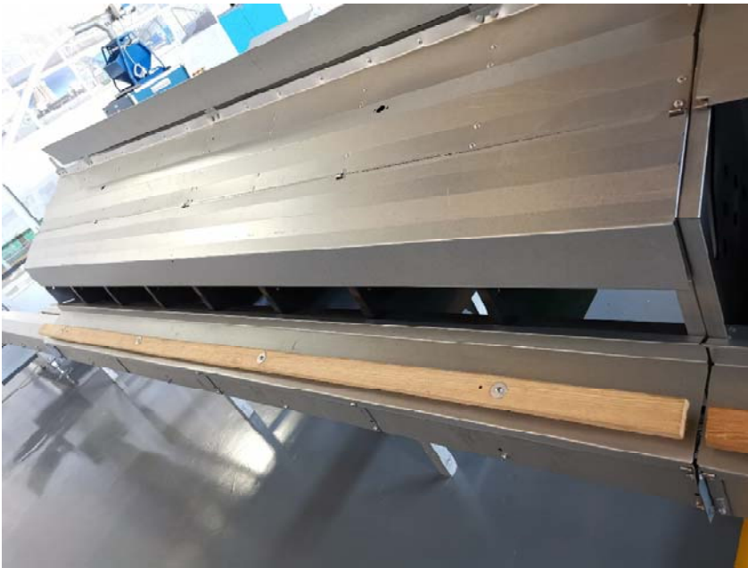
High quality sylphard pine pedal is installed above the egg belt
